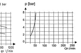
Hysteresis of  $\mathbf{p_2}$  as a function of rising (falling) **p**<sub>1</sub> at a constant draw-off rate QN 20 l/min Basic setting (starting point): p<sub>1</sub>: 7.0 bar p<sub>2</sub>: 2.0 bar
