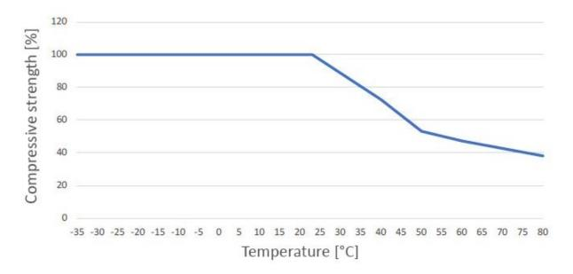
The degree of utilisation of the permissible compressive strength (%) as a function of the temperature (°C). These specifications are valid for the operating medium air.
