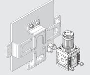
The bracket can be secured in any position, and the fittings can be mounted on the pressure gauge air intake at the back of the unit.
